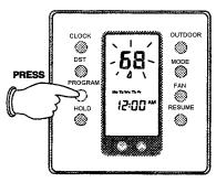
Step 5: Press the DECREASE button or INCREASE button to set the desired minutes for the Morning " " " event (program starting times are set in ten-minute increments).
